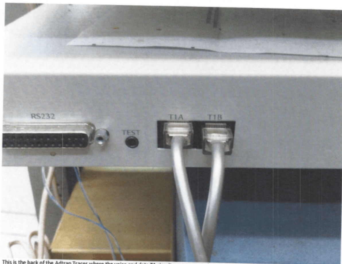
This is the back of the Adtran Tracer where the voice and data T1 circuits are connected. T1A connects to the voice jack (the upper one on the board in the image above) and the data jack connects to T1B.
